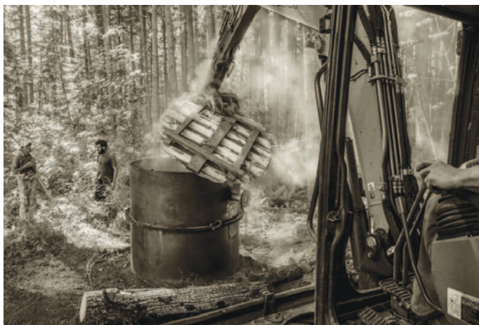
Here is the author using the cylinder burn method for making biochar using a 5' by 5' metal cylinder cut from a water tank.
